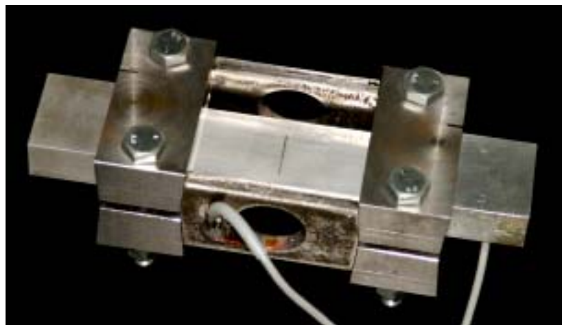
Figure 2: Photography of a specimen installed in the loading equipment. The loading is applied by a simple torque wrench on 4 screws.
